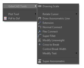
**Cross to Break:** In engineering drawings, many places need to break the cross line. If we do this in the original way, it will be very complex. Using this function to break lines can be easily done.
