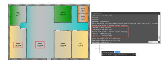
**Total length:** Calculates the object length and total length associated with selected arc, circle, polyline segments or line objects. You can either select the single object by clicking or selecting multiple objects with window selection.
